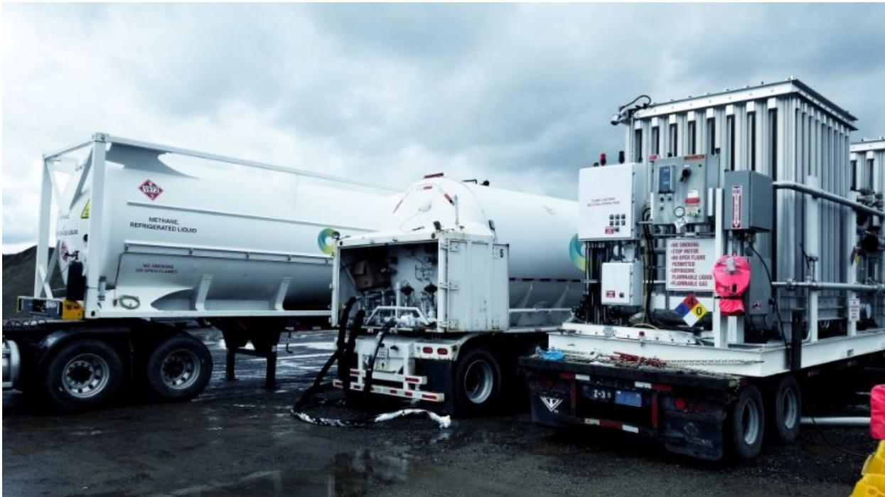
CLEANCOR's mobile equipment packages are designed to let an asphalt plant temporarily operate on LNG while the plant is being permanently transitioned to LNG as its fuel source.
